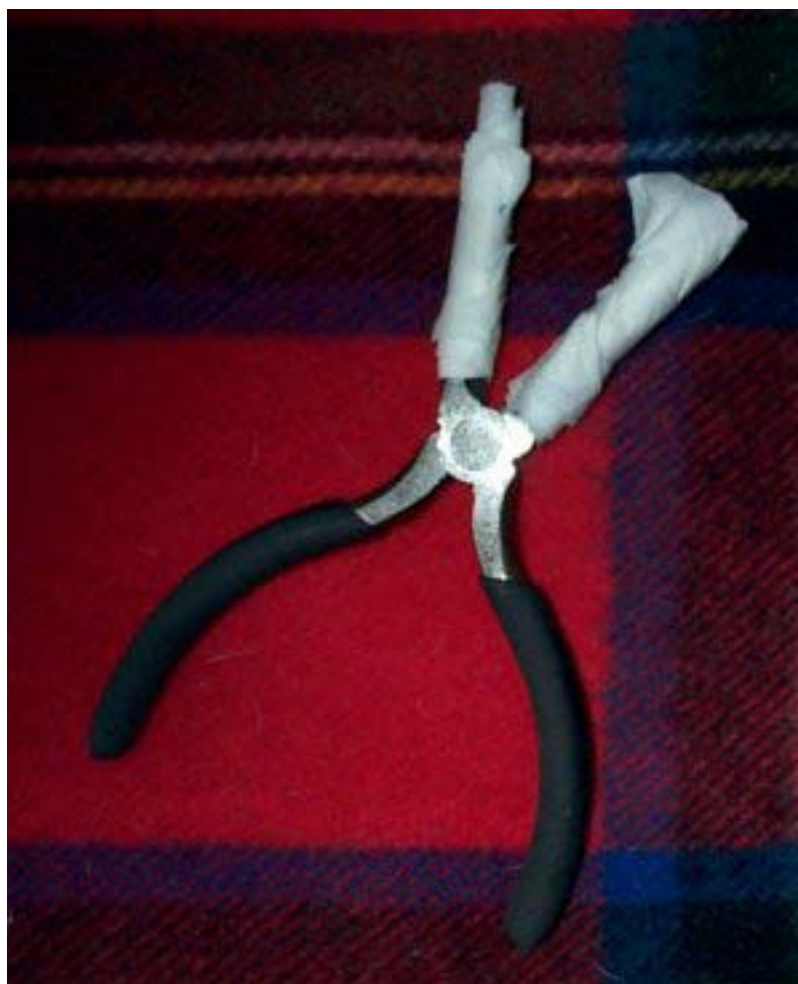
Figure 1 – my pliers, with the jaws covered in many layers of paper towel so they won't damage the knobs if I need to use the pliers to remove them. (In the end, four knobs had to be removed this way)
