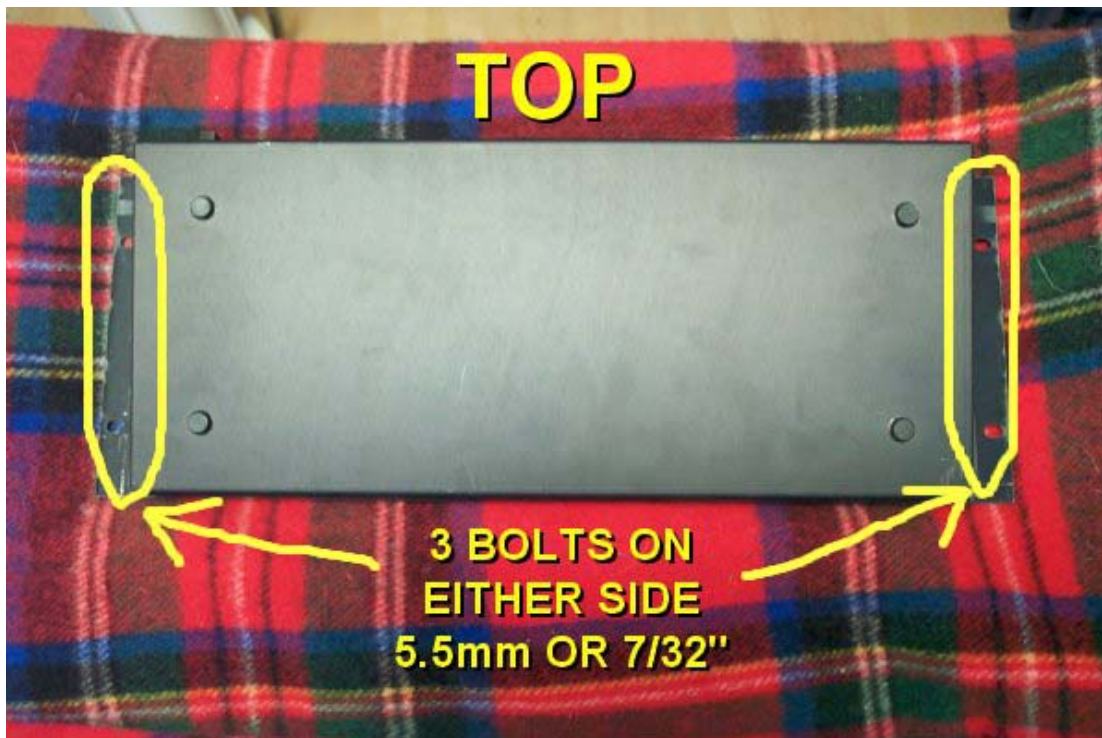
Figure 2 – the underside of the Bitstream Pro prior to removal
